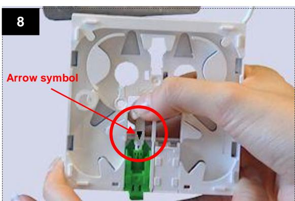
Thread the DiaLink through the opening from back to front and put it into the adapter. Be sure that the black arrow symbol is at the top and is fed into the adapter's guide groove.
