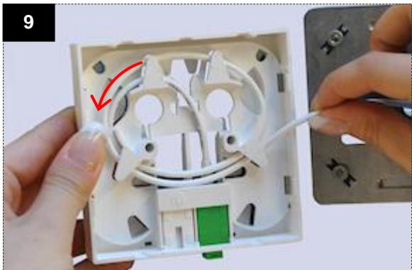
Flip the socket over and carefully wind the cable around the cable pins, two times to the left.
