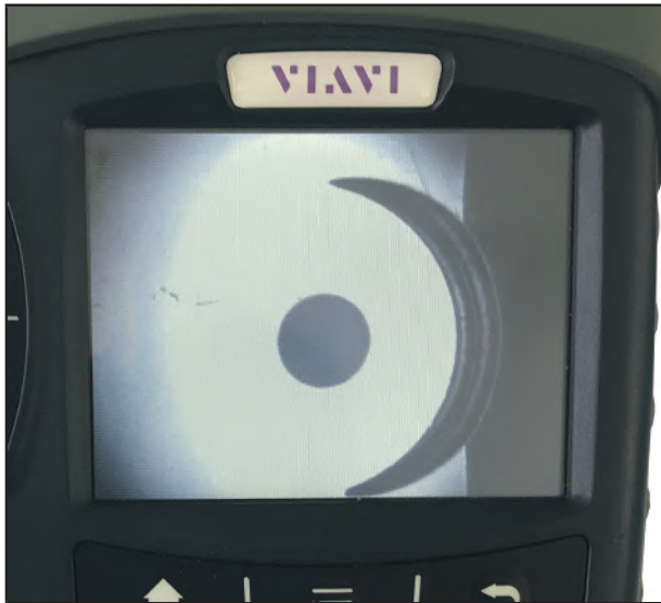
Accepted – clean end face (100X magnification )
