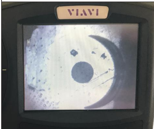
Not accepted - dirt on the end face (100X magnification)
