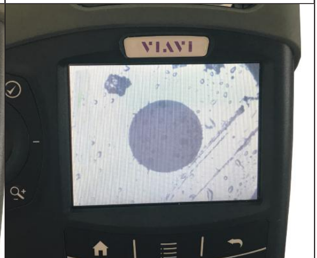
Not accepted - dirt on the fibre (200X magnification)
