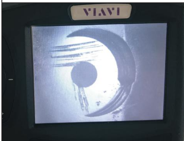
Not accepted – scratches after cleaning (100X magnification)
