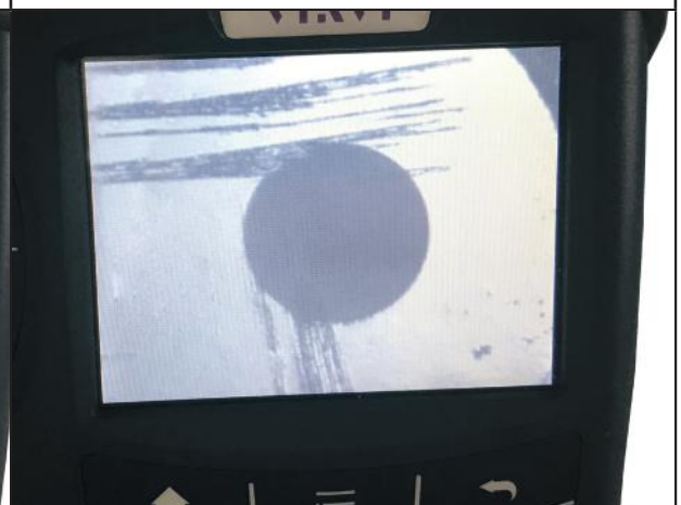
Not accepted – scratches after cleaning (200X magnification)
